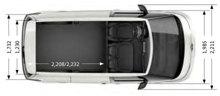
Please note: Vehicle drawings are not to scale. All dimensions in millimetres (mm), unless otherwise stated. The height measurements listed may vary by  $\pm$  40mm depending on model and equipment fitted.
